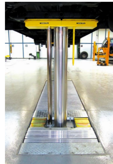
Telescopic ram with an optional safety bar (conforming EN 1493:2010)
