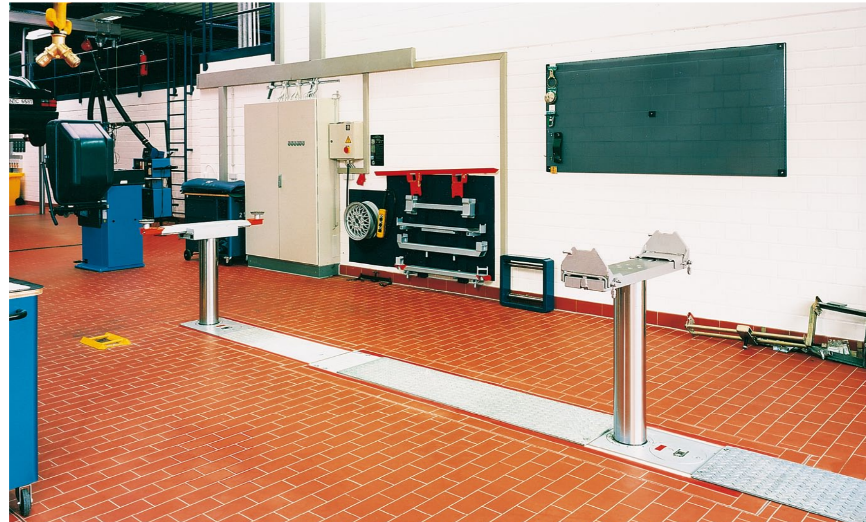
Photo: two-ram-lift Lifting capacity 8.000 kg per lifting ram
