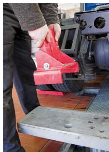
Exchangeable support system for lifting of diverse vehicle types.
