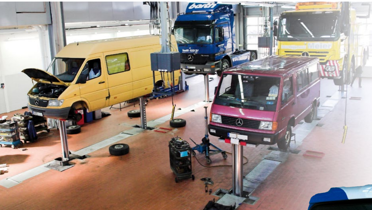
2 HVV four-ram-lifts, which are used as 2 two-ram-lifts.
